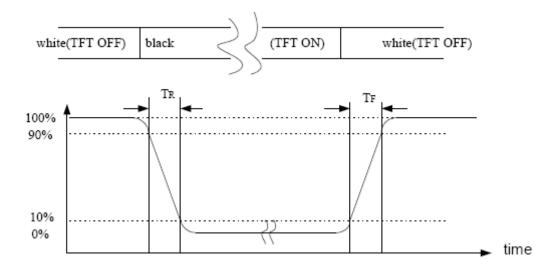
Note 4: Definition of optical measurement setup
